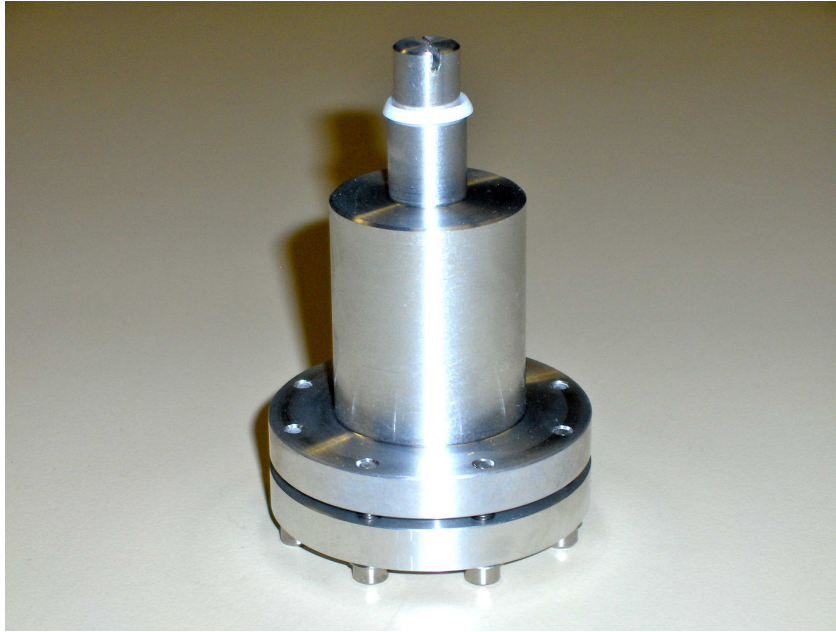
Figure 6.2.: The photo depicts the scintillator container that was used for the light yield measurements. It has been made of aluminum due to its high reflectance.
