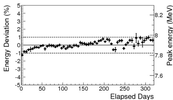
Mean energy of the Gd-neutron capture peak in the Double Chooz Target liquid as function of elapsed days [2]
