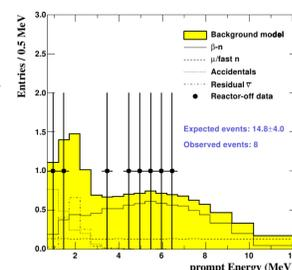
Energy spectra of the various background contributions measured during 7.5 days reactor off, confirming the predicted rates
