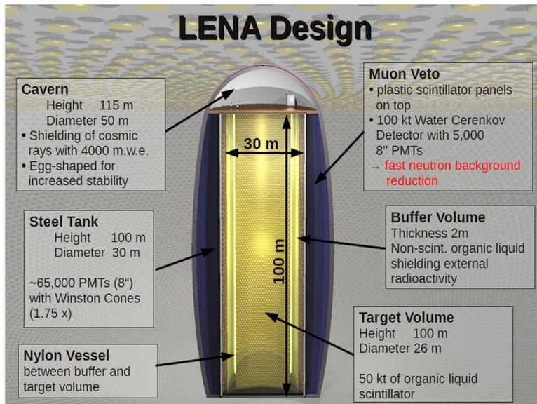
Fig. 5. Schematic view of the LENA detector with about 50 kton active liquid scintillator mass.
