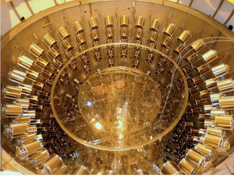
Fig. 2. Photo of the Double-Chooz far detector after installation of the acrylic vessels.
