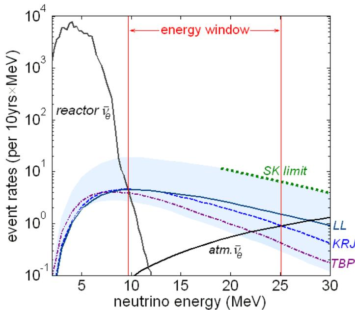
Fig. 6. Event rates of reactor, atmospheric and DSNB  $\bar{\nu}_e$  (according to three different models) as expected for LENA in Pyhäsalmi after ten years of measurement. The shaded region represents the possible range of the DSNB rates depending on the normalization of the SN rate. The Super-Kamiokande limit is indicated.
