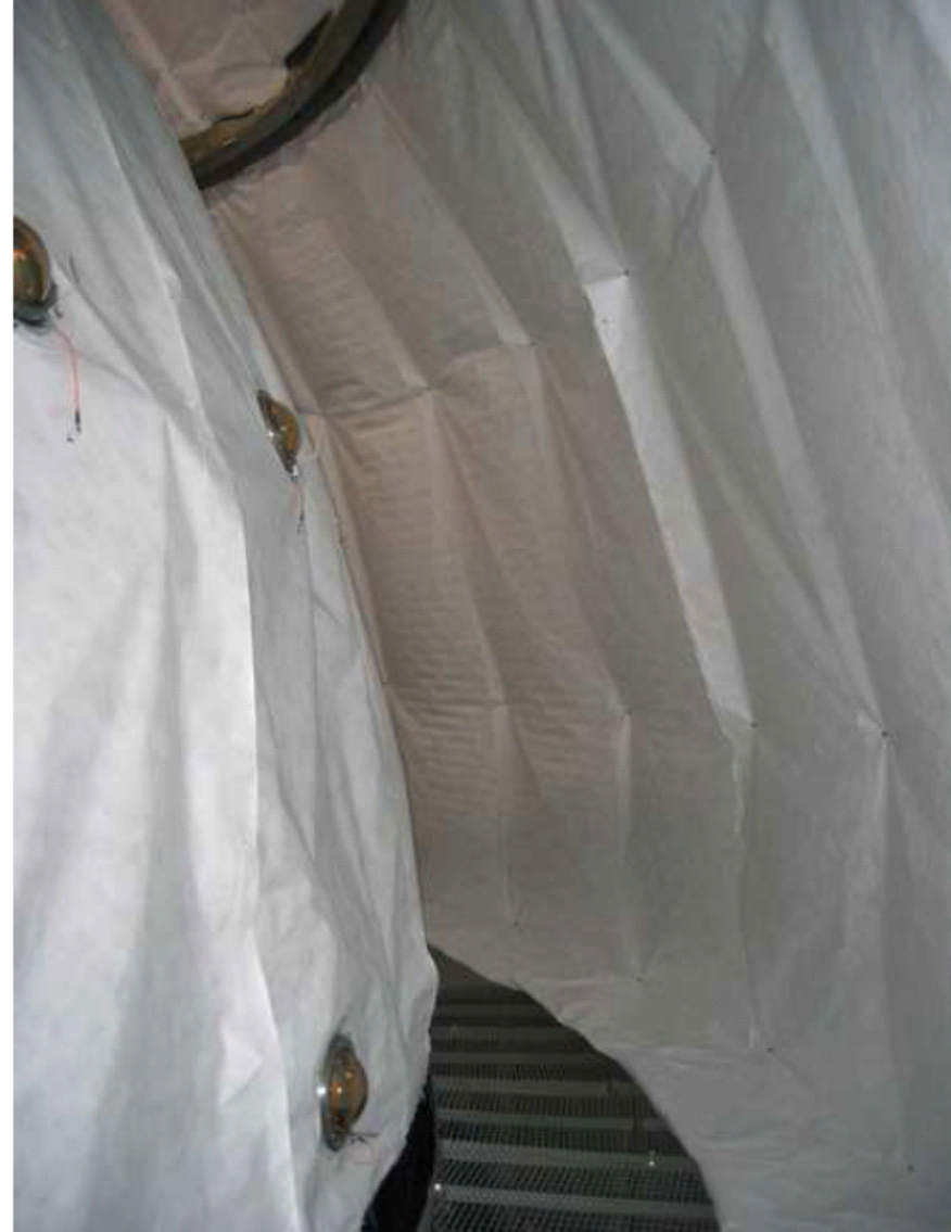
Fig. 5. The inner surface of the Water Tank covered with a layer of Tyvek. The Tyvek sheets improve light collection in the Outer Detector by reflecting the photons back into the water.
