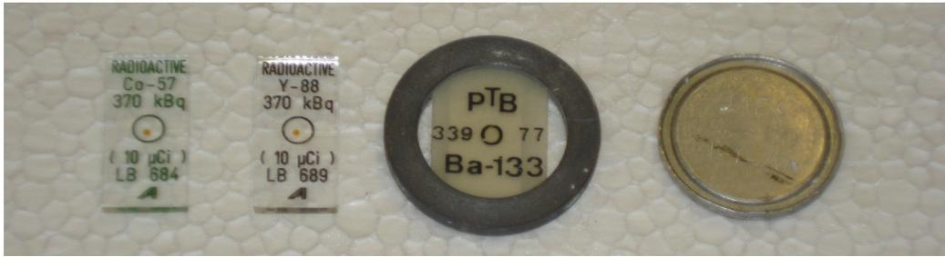
Figure 4.3: Calibration sources used for measuring the detector efficiency. From left to right:  $^{57}\text{Co}$ -source,  $^{88}\text{Y}$ -source,  $^{133}\text{Ba}$ -source and  $^{60}\text{Co}$ -source. The radioactive material is a small metallic dot in the centre of each calibration source (only visible for  $^{57}\text{Co}$  and  $^{88}\text{Y}$ ). The size of the  $^{60}\text{Co}$ -source is nearly the same as an 1 Euro coin.
