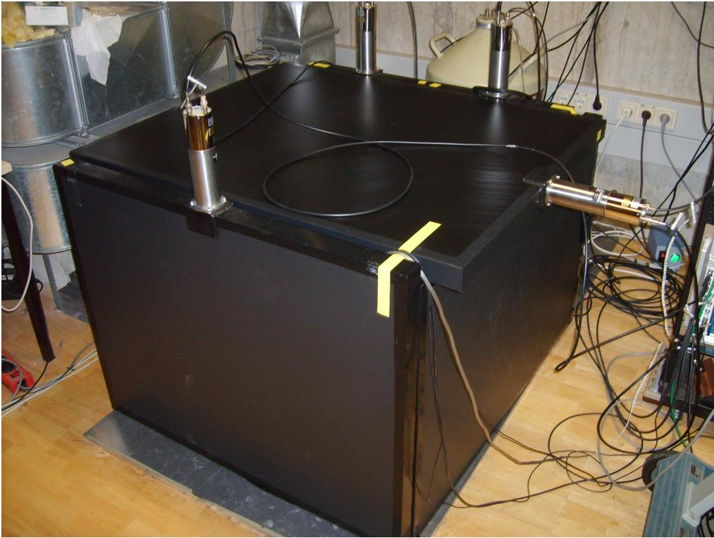
Figure 3.9: *The fully equipped active muon-veto system consisting of 6 plastic scintillator panels with photomultiplier tubes. The panels are made of a scintillating material called BC408, which is based on polyvinyl toluene (see fig. 3.10).*
