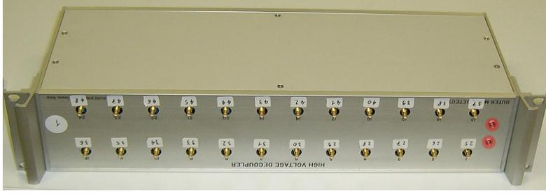
Figure 3.3: Front-end side of a *High Voltage Decoupler* (HVD) frame, upside down. A pulser signal can be injected into both boards of the HVD via the newly installed *Pulser System Connectors* (PSC) (marked in red).
