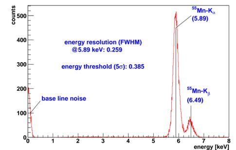
$^{55}\text{Mn}$  x-ray spectrum recorded with 0.8 g detector (see left picture). Separation of the Mn- $K_\alpha$  and Mn- $K_\beta$  line can clearly be seen. Energy threshold: 0.385 keV, resolution @ 5.9 keV: 0.259 keV
