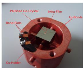
Cryogenic detector with 3.2 g germanium absorber
