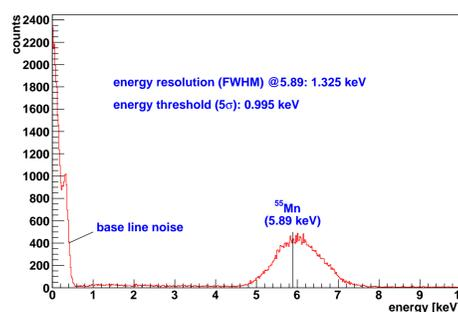
$^{55}\text{Mn}$  x-ray spectrum recorded with 3.2 g detector (see left picture). Energy threshold: 0.995 keV, resolution @ 5.9 keV: 1.325 keV
