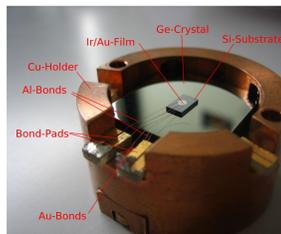
Composite detector with germanium absorber
