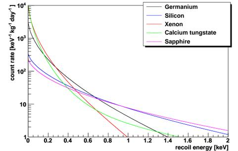
Recoil spectra of reactor neutrinos for different target materials
