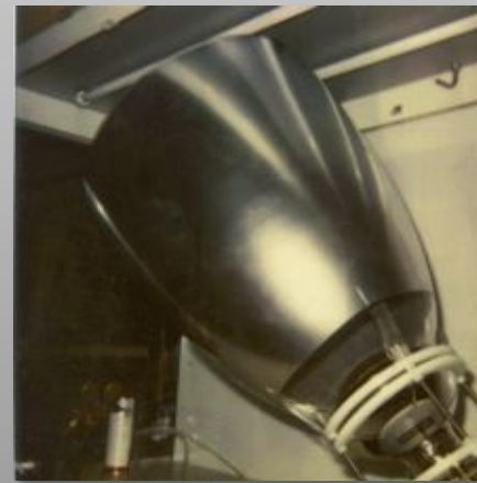
Light cone used in the Borexino prototype CTF, eight-fold light collection
