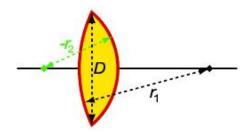
$$f = \frac{1}{n-1} \frac{r_1 r_2}{r_2 - r_1} = 79.8 \text{mm}$$
