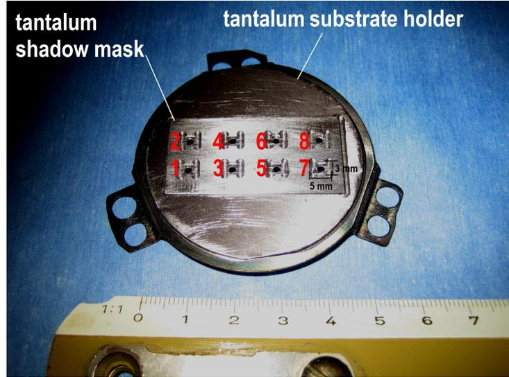
Figure 6.1: Tantalum shadow mask used for the production of the "small" sputtered tungsten thin films. The substrate holder with the exchangeable shadow mask can be seen. The positions for the eight substrates are shown, corresponding to the film numbers of the produced film (see section 6.3). One cutout can accommodate a substrate of  $3 \times 5 \text{ mm}^2$ . The unsealed area for each film is given by a circle with a diameter of  $\sim 2 \text{ mm}$ .
