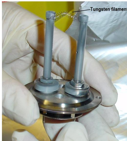
Figure 4.4: Tungsten filament of the ion source. The length of the filament is 2 cm.
