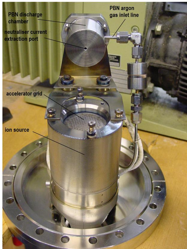
Figure 4.6: Complete setup of the ion source together with the plasma bridge neutraliser. On top of the ion source the acceleration grid can be seen. The PBN discharge chamber is mounted above the ion source.
