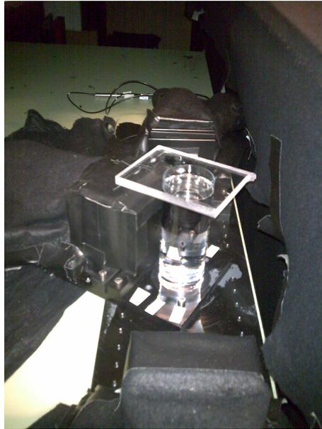
Figure 6.6: *A photograph of a sample in the experimental setup. In the foreground there is the LED and the interference filter which is covered with felt. Then, the sample can be seen which is filled into a cylindrical glass and covered in order to keep it clean from dust particles. To the left, the PMT that detects the scattered light is covered with felt, as is the PMT in the background which detects the light that passed the sample.*
