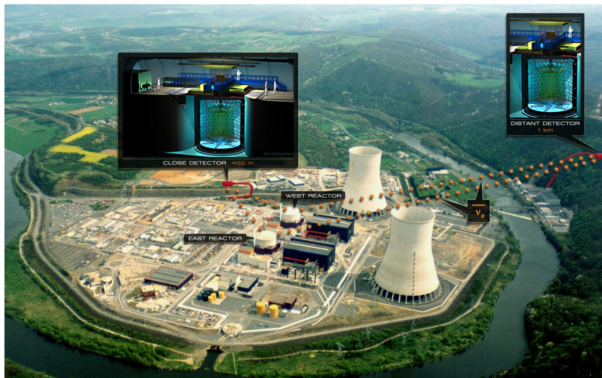
**Figure 2.1:** *The Chooz reactor site and the positions of the near and far detector of the DOUBLE CHOOZ experiment [Irf10].*
